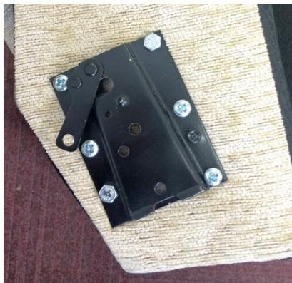
The “locking” bracket in the “unlocked” position.
